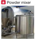
Jsed for mixing powder such as milk, cocoa, sugar and stabilizers with milk or water, for the process of: reconstructed milk, flavoured milk, yogurts, ice cream and others. Available in sizes of 500, 1,000 &
