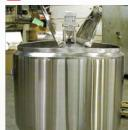
For pasteurized milk storage, yogurt and sour cream fermentation, cheese coagulation and ice cream ageing. The tanks are with an insulated layer and can have a double lacket for heating or cooling, agitator with gearmotor and drain butterfly valve. Sizes are from 400 up to 5,000 liters
